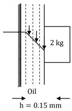
If interface area of block is  $0.04 \text{ m}^2$ , it's dynamic viscosity is  $7 \times 10^{-3}$  pa-sec. Find out the terminal velocity of the block.
